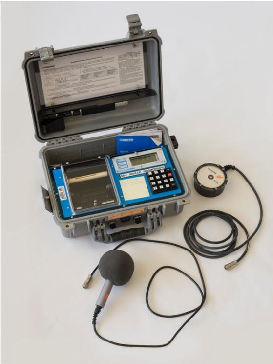
The portable seismograph system—usually set up at a house—records ground vibration and sound (airblast) from blasting events. The seismograph system includes:
