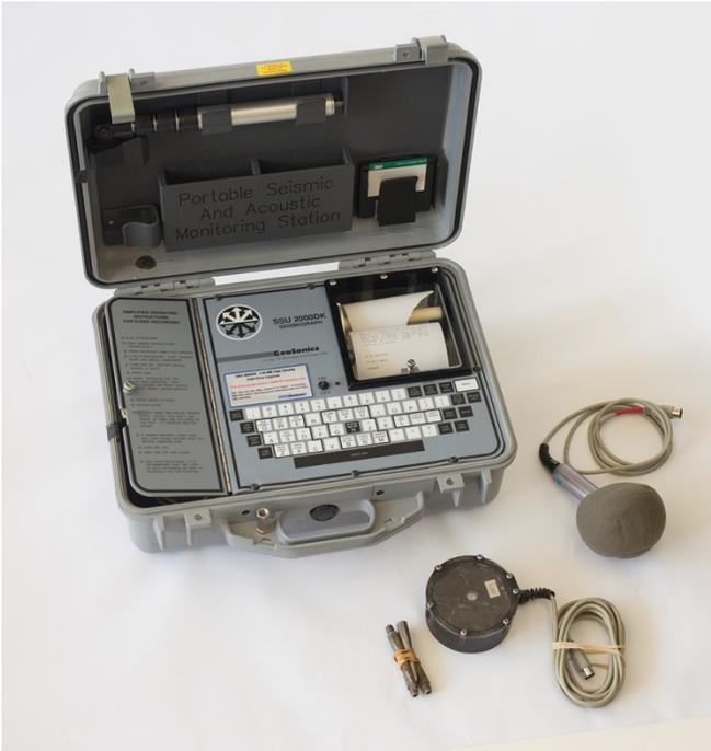
The portable seismograph system—usually set up at a house—records ground vibration and sound (airblast) from blasting events. The seismograph system includes:
