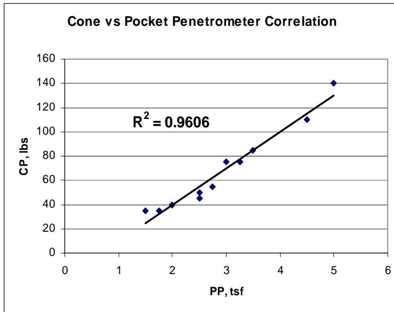
Figure 15. Comparison of cone penetration and pocket penetration strength measures for near surface uplands samples from all study subwatersheds.
