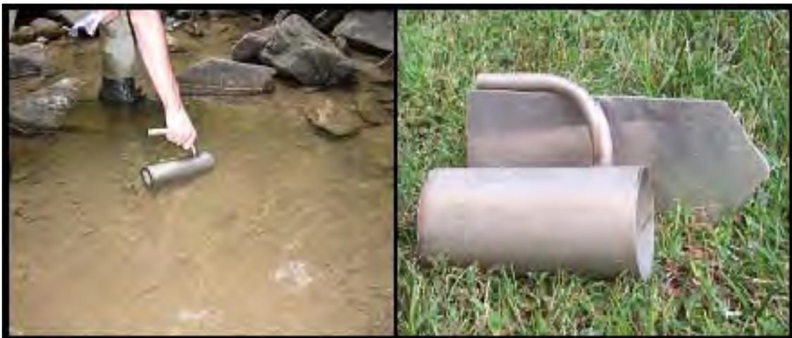
Figure 9. Modified McNeil sediment sampler (McNeil and Ahnell 1960; Williams 2005).
