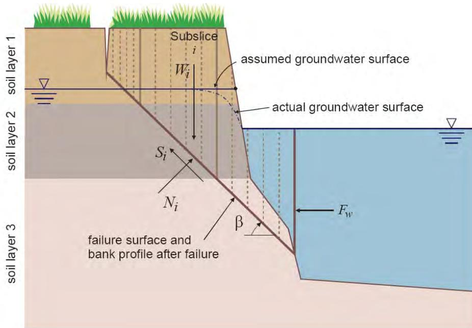
Figure 5. Summary of forces on a failure block used in ConCEPTS bank stability analysis (from Langendoen 2000).
