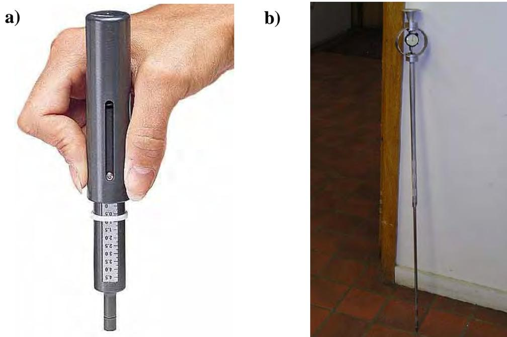
Figure 16. Illustration of a) Cole Parmer model EW-99039-00 pocket penetrometer, and b) Hogentogler model S-4615 cone penetrometer.
