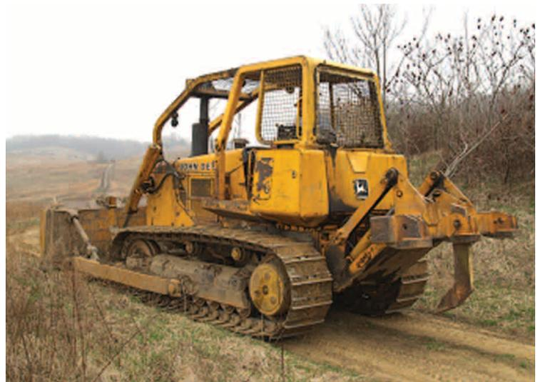
ABOVE PHOTO: D-6 sized dozer equipped with 36-inch ripping bar.
