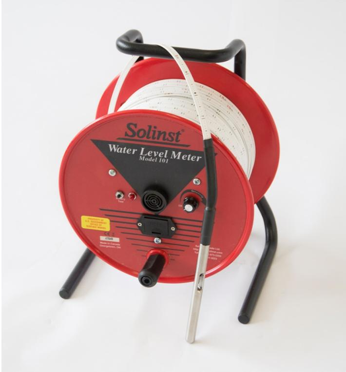
The water-sensing probe is attached to a 300-foot polyethylene flat tape with permanent markings every 1/100 of a foot. A dial allows the buzzer to be adjusted or turned off when the probe is in cascading water and ensures a clear signal when the probe contacts high- or low-conductivity water. The tape is wound on a 10-inch diameter plastic reel with a brake.
