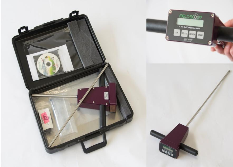
The portable soil compaction meter uses a cone penetrometer to measure soil compaction to a depth of 18 inches. The unit has a datalogger function that allows measurements to be downloaded to a computer. The unit can also log GPS location using a Bluetooth connection to an appropriate GPS unit.
