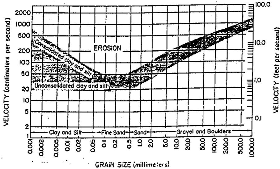
Hjulstrom's diagram, showing critical velocity for movement of quartz grains on a plane bed at a water depth of one meter, as modified by Sundborg (1956). The shaded area indicates the scatter of experimental data. There are very few reliable data in the clay and silt region.
