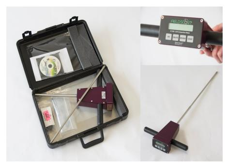
The portable soil compaction meter uses a cone penetrometer to measure soil compaction to a depth of 18 inches. The unit has a datalogger function to allow collection of sets of data that can be downloaded to a computer. The unit can also log GPS location using a Bluetooth connection to an appropriate GPS unit.
