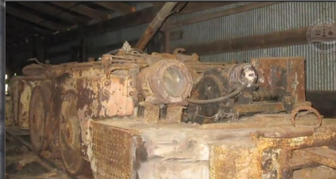
Photo: The old train engine that was used to move coal from inside in the underground mine at the Dessecker Mine in Ohio.
