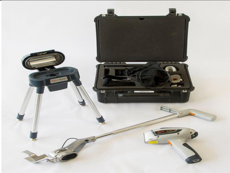
**Description:** The Niton XL3t 950 GOLDD+ handheld analyzer is a portable elemental analysis tool that will detect elements with an atomic number 12 or above and will present a spreadsheet with the measured elements in either parts per million or as a percentage of the material being tested.
