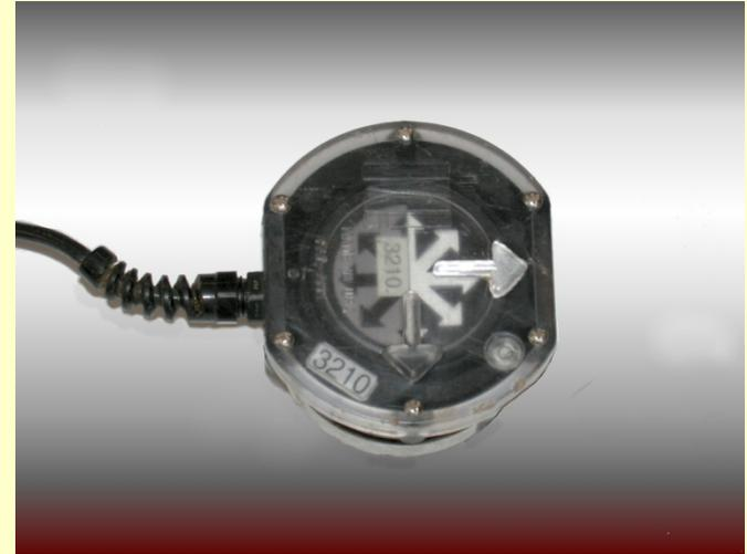
Where access to the structure and/or property is not available, the sensor should be placed closer to the blast in undisturbed soil.
