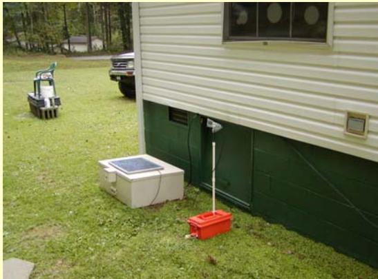
If placed too close to a structure, the airblast may reflect from the house surface and record higher amplitudes. Structure response noise may also be recorded. Reflection can be minimized by placing the microphone near a corner of the structure. (RI 8508)
