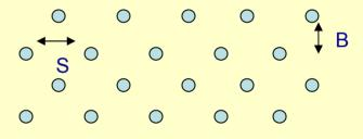
A staggered blast pattern is used for row firing, where the holes in one row are fired before the holes in the row immediately behind them. The square and rectangular blast patterns are used for firing "V" (chevron) or echelon rounds.
