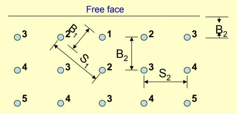
Numbers indicate firing sequence ( $B_1$  = true burden;  $B_2$  = apparent burden;  $S_1$  = true spacing;  $S_2$  = apparent spacing).
