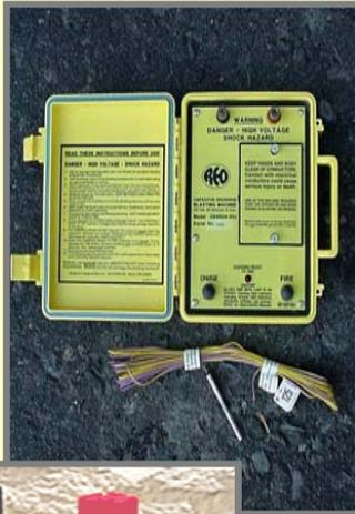
The lead (firing) line should not be laid out until the blast circuit is completely wired and all unnecessary personnel have been cleared to a safe location. After the lead line is laid out, it should be tested with a blaster's multimeter for continuity.
