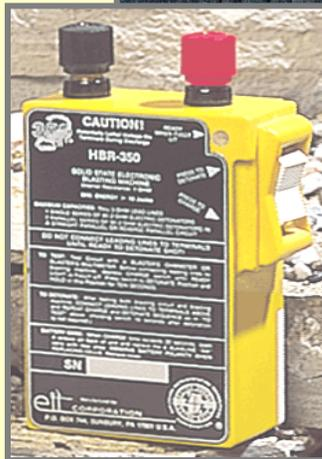
The lead line must be shunted at the blasting machine before connecting the other end to the blasting circuit. **NEVER** connect an unshunted lead line to the blasting circuit.
