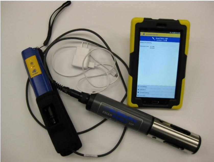
The smarTROLL MP handheld instrument has a combined pH/ORP sensor and other sensors for temperature, conductivity, pressure, and dissolved oxygen.
