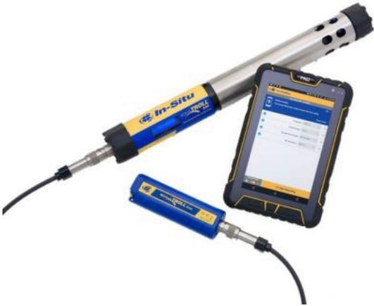
The AquaTROLL 500 MP handheld instrument has a combined pH/ORP sensor and other sensors for temperature, conductivity, pressure, and dissolved oxygen. The completely submersible sensor-equipped probe is connected to the rechargeable power pack. Sensor readings are transmitted by Bluetooth from the power pack to the Android or iOS tablet/smart phone. The unit uses In-Situ's VuSitu app to collect the data.
