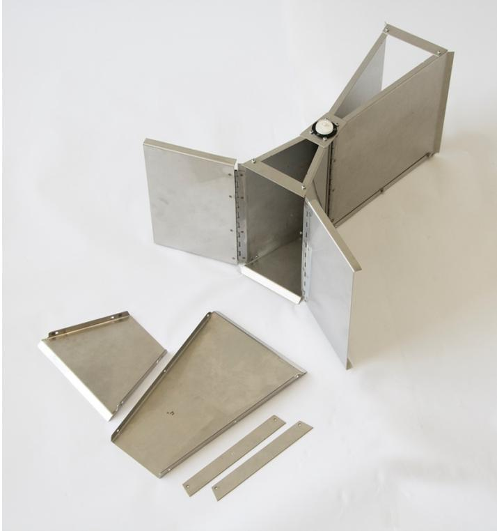
This stainless steel, flat-bottom flume can be disassembled for easy transport. It can be set up with either a one-inch throat (2.5–125 gpm) or four-inch throat (10–250 gpm). The unit comes with entrance wing walls to divert flow into the upstream converging section of the flume.
