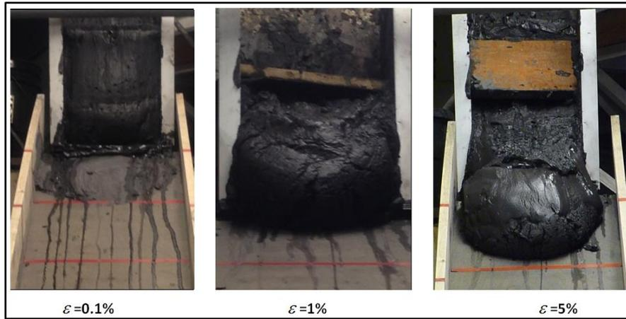
**Figure 2: Results of impact loading tests (at different strains  $\epsilon$ ) on KY sample under different compressive strains ( $\alpha = 30^\circ$ ,  $w=48\%$ )**
