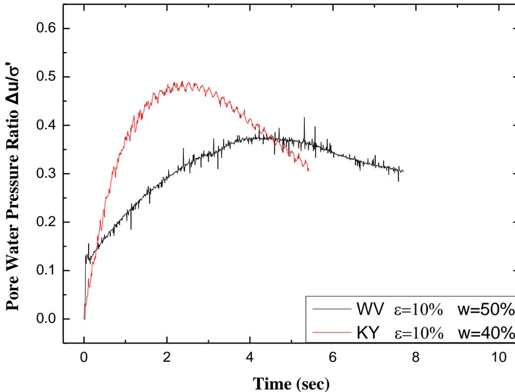
**Figure 4: Recorded pore water pressures in slurry cells under impact loading.**
