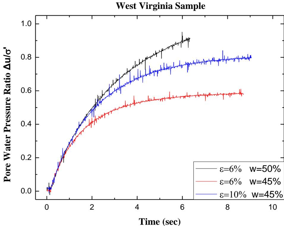
**Figure 3: Recorded pore water pressures under impact loading.**
