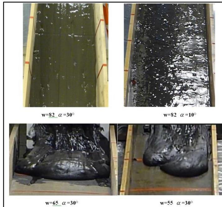
**Figure 1: Flows of the WV sample at different water contents (w) and slope angles (α).**
