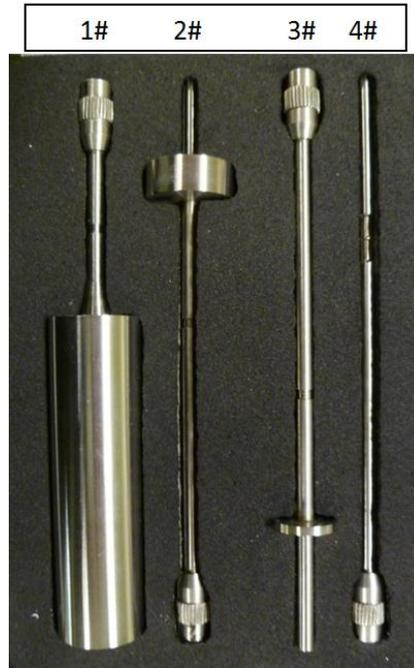
Figure 2-33 Four types of spindles of NDJ-8S digital rotary viscometer
