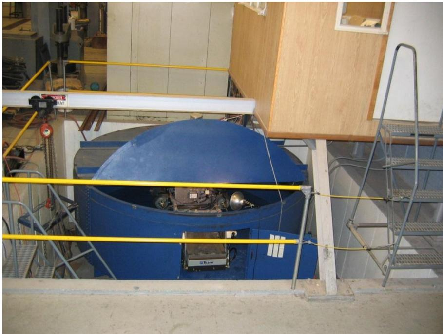
Figure 4-2 CWRU geotechnical centrifuge
