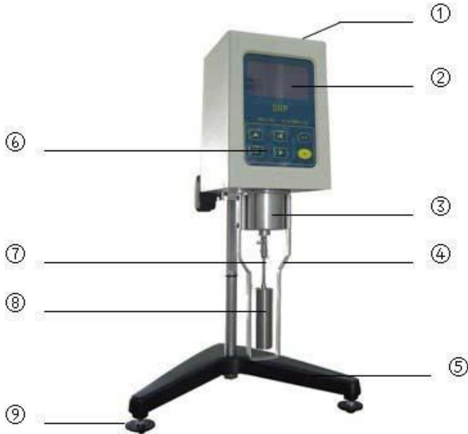
Figure 2-32 Structure of NDJ-8S digital rotary viscometer: (1) Level indicator (2) Display Screen (3) Housing (4) Protection bracket (5) Base (6) Operation key (7) Rotor connector (8) Rotor (9) Level adjustment knob
