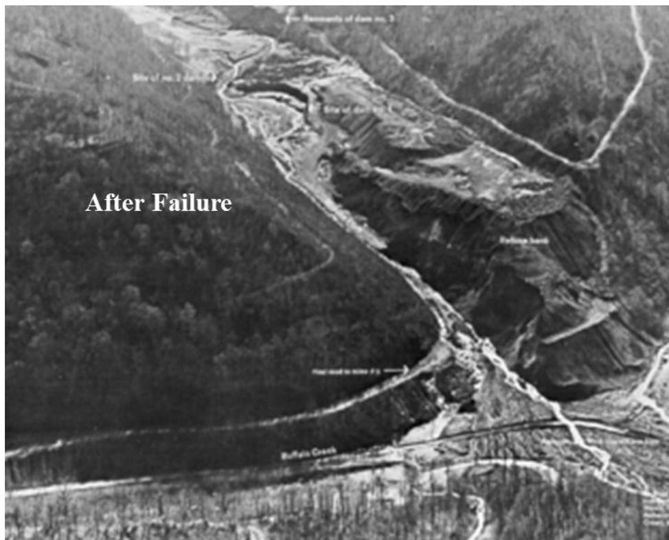
Figure 1-4: Failure of impoundment in Buffalo Creek area
