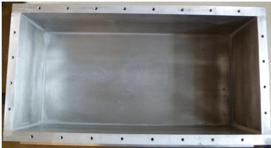
Figure 4-4 Rigid box on the CWRU geotechnical centrifuge
