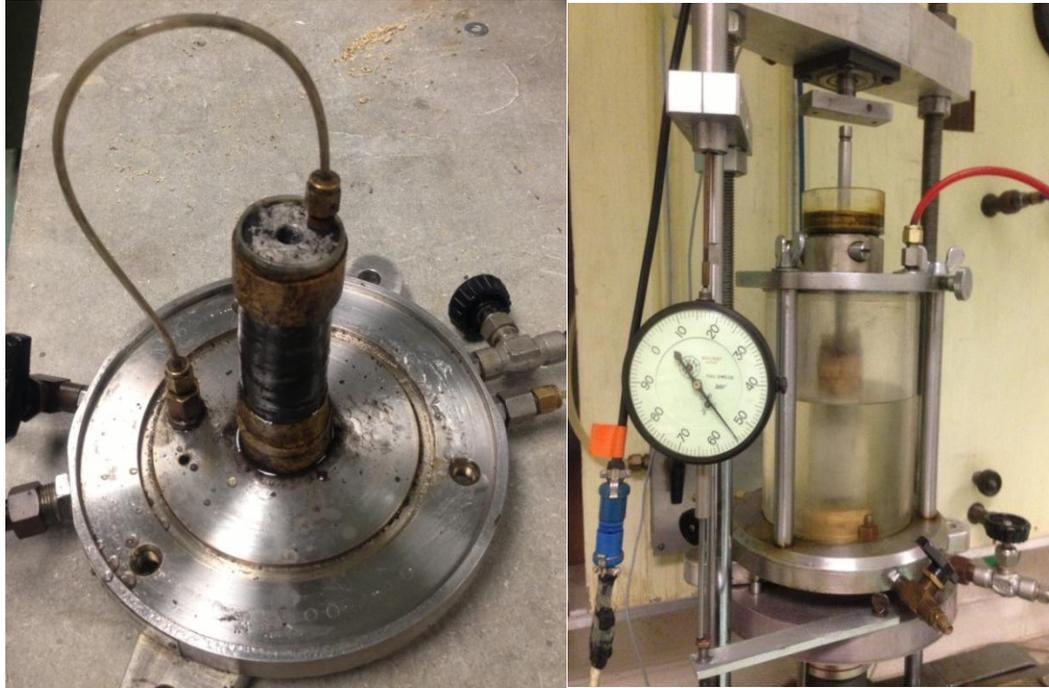
Figure 2-23 Prepared test sample and triaxial chamber for triaxial tests
