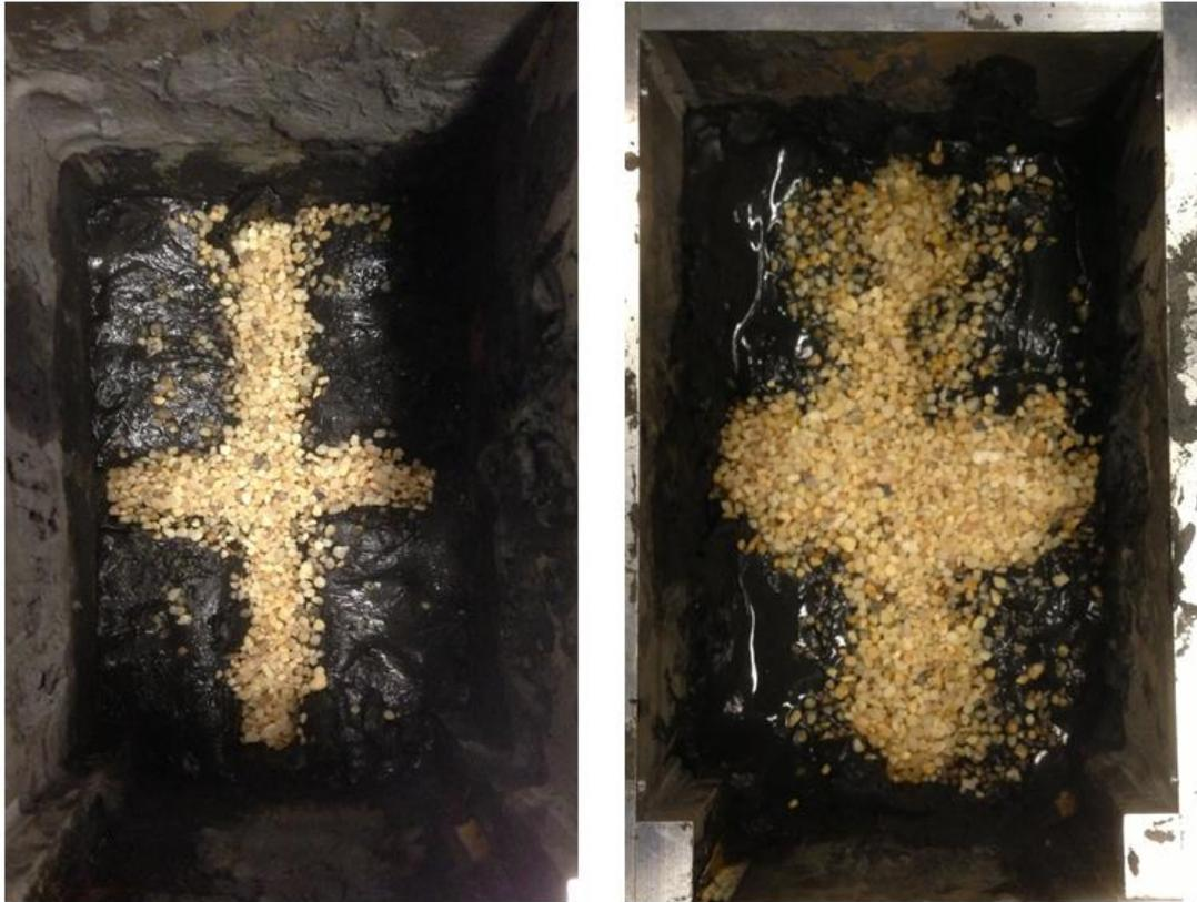
Figure 4-15 Centrifuge model with coarse refuse build cells
