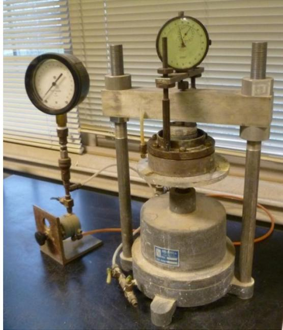
Figure 2-9 Consolidometer used in consolidation test
