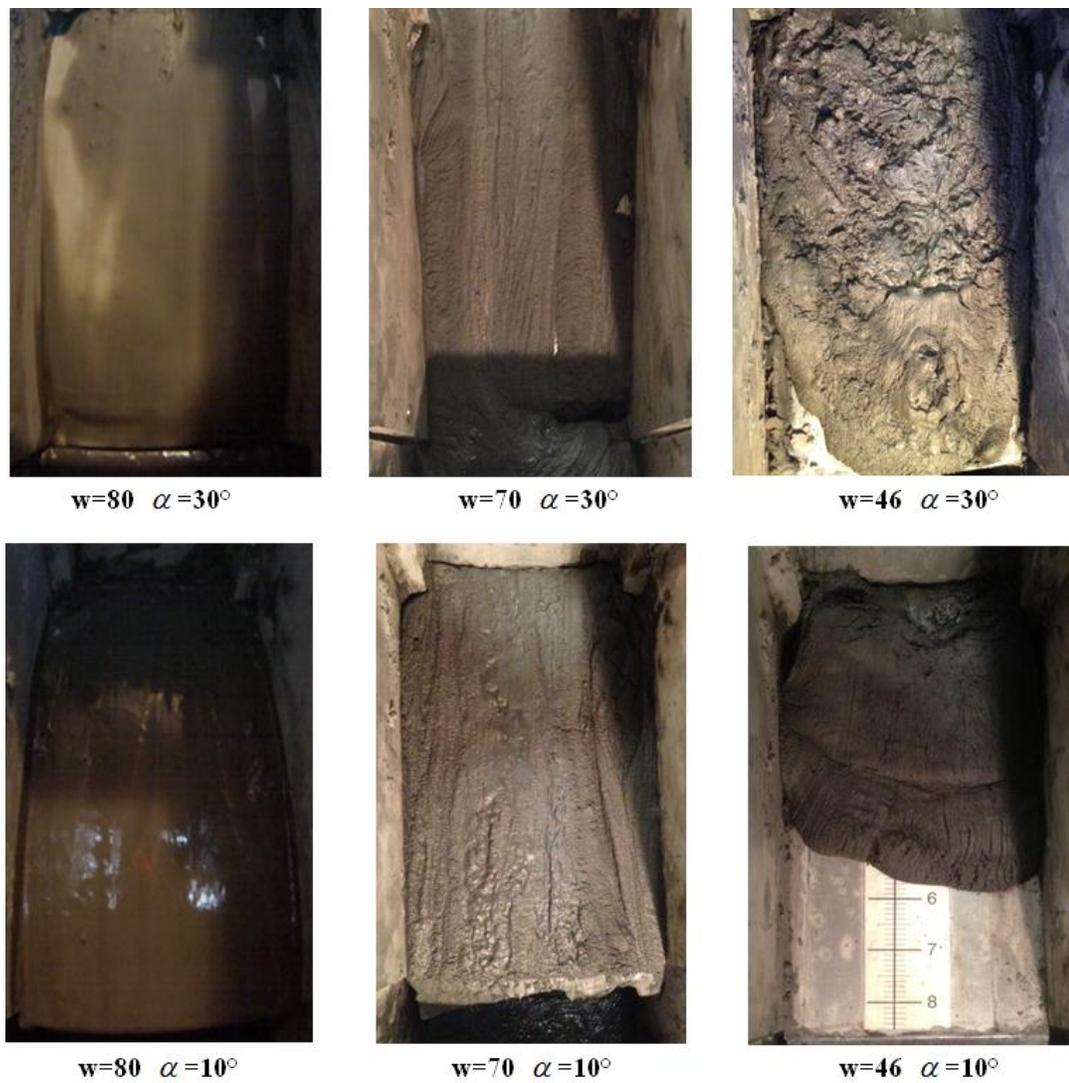
Figure 4-10 Flow of KY coal refuse sample in the centrifuge tests
