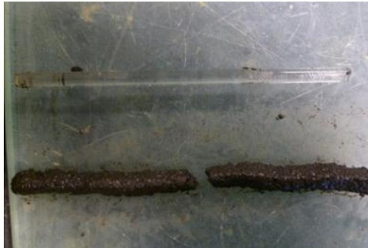
Figure 2-6 Plastic limit test on coal refuse sample
