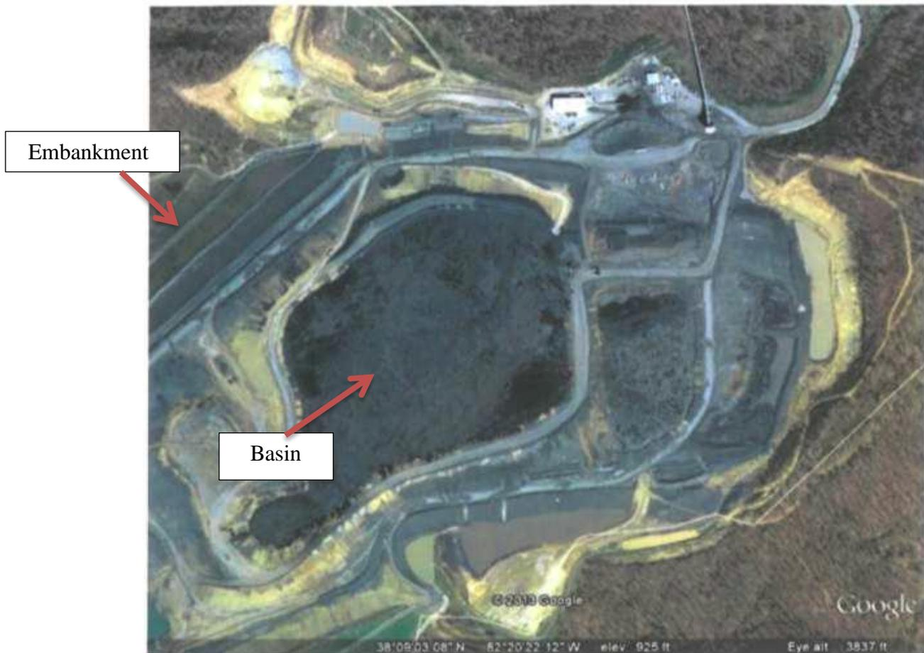
Figure 1-1 Overview of a typical coal waste slurry impoundment
