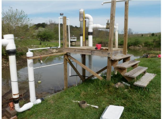
The test trompe apparatus included adjustable outlet pipe (uppipe), and clear horizontal separation chamber and air induction head piping. Various air tube configurations and 2", 3" and 4" downpipes were tested over a range flow rates.
