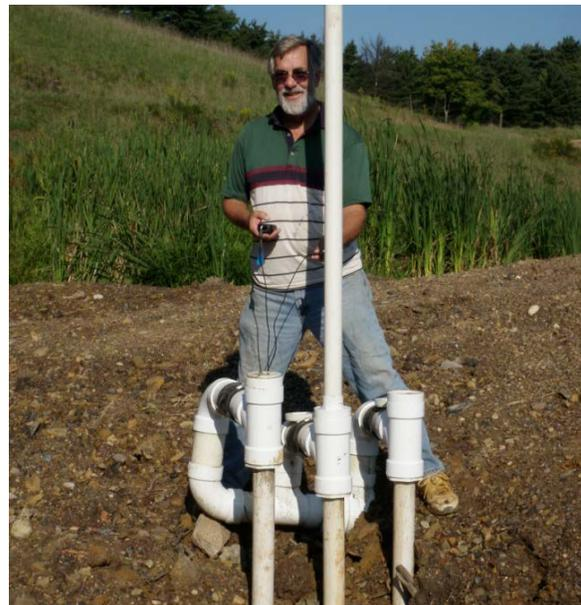
Bruce Leavitt, PE, PG uses an anemometer to measure volume of air being compressed by the demonstration trompe at the North Fork Montour Run passive treatment system. Pictured is the inlet of the first of three triple-inlet trompes installed in series.
