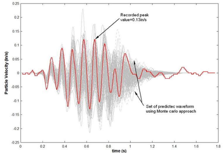
FIGURE 1: Improved Signature methodology and actual reading.
