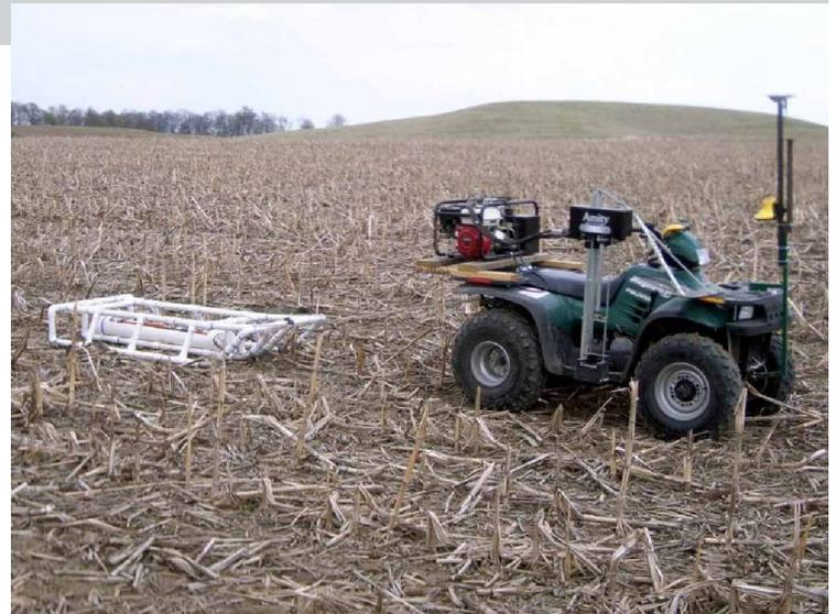
ABOVE PHOTO: Collection of terrain and electrical conductivity measurements at the Lewis Mine site in Indiana.
