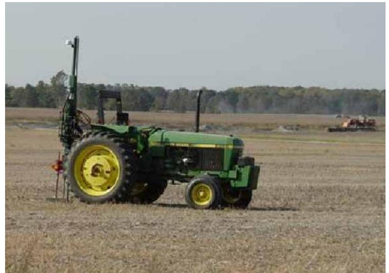
ABOVE PHOTO: Collection of cone penetrometer test measurements at the Lewis Mine site in Indiana.
