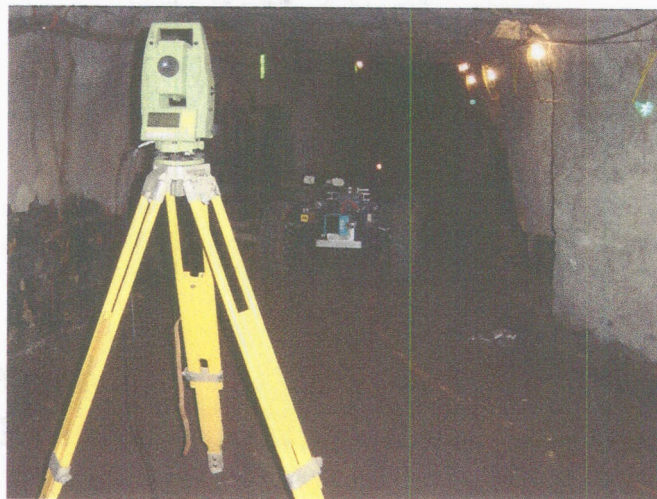
Figure 6: Automated survey instrument tracking CaveCrawler in the Research Mine
