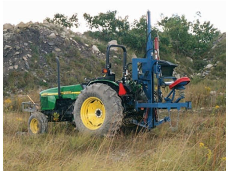
ABOVE PHOTO: This is a photograph of the Static Cone Penetrometer.
