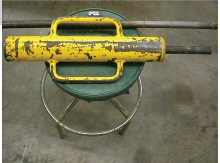
ABOVE PHOTO: This is a photograph of the Dynamic Cone Penetrometer.
